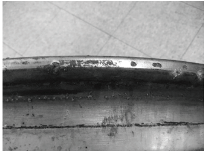
Picture 13-37 Acceptable pitting
