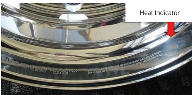
Picture 13-2 Heat Indicator at wheel flange
